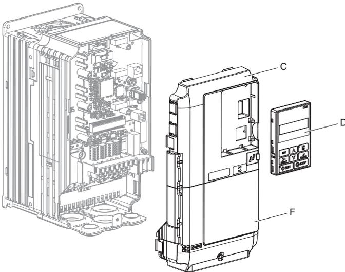
Figure 3 Remove the Front Covers and Digital Operator
