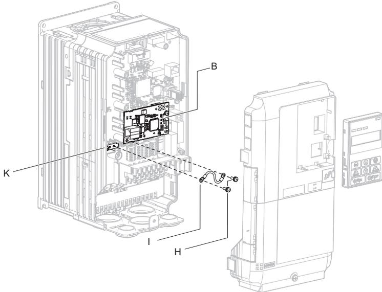
**Figure 6 Connect the Ground Wire**
