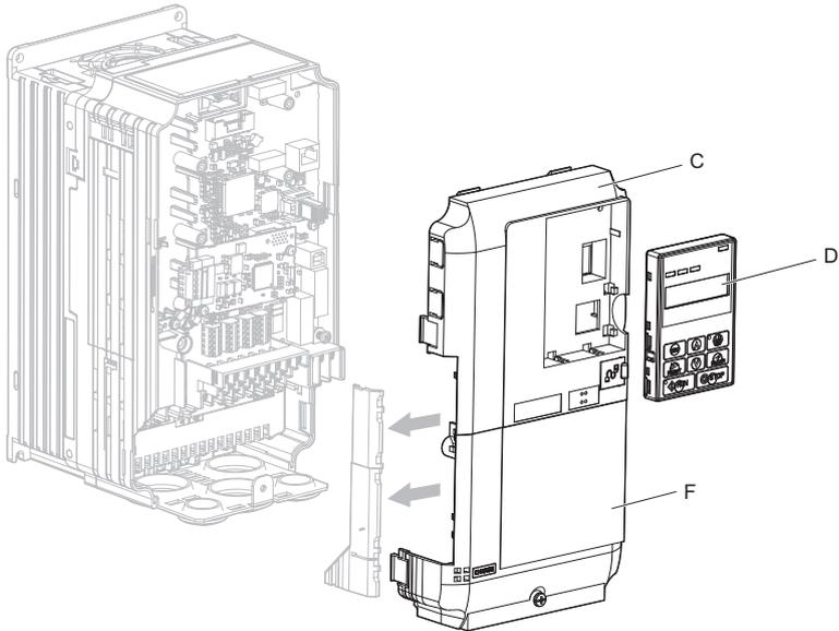
**Figure 9 Replace the Front Covers and Digital Operator**
