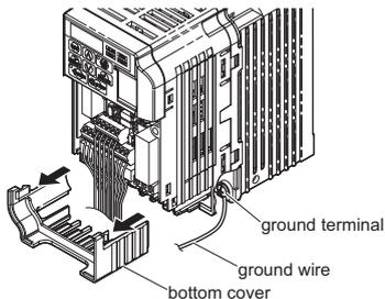
**Figure 8 Connect Ground Wire**
