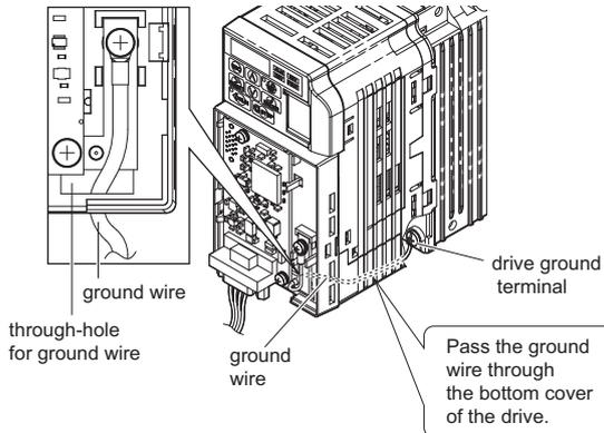
**Figure 12 Ground Wire Connection**
