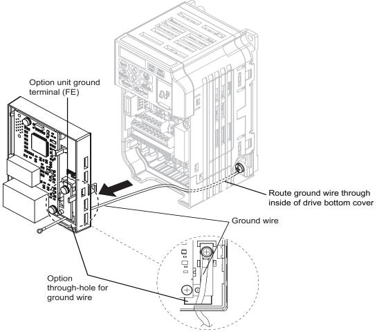
Figure 21 Ground Wire Routing
