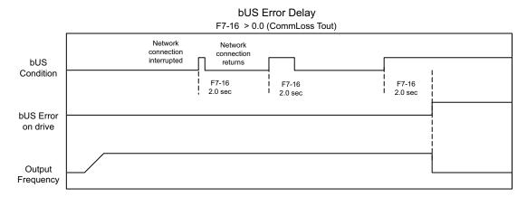
Figure 54 bUS Error Delay Timing Example
