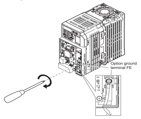
Figure 23 Connect the Ground Wire to the Option
