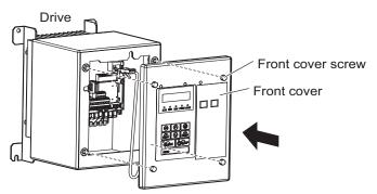
Figure 38 Attach Cover to Drive
