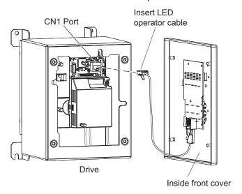
Figure 37 Insert LED Operator Cable to Drive CN1 Port
