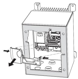
Figure 27 Remove the Lower Terminal Cover
