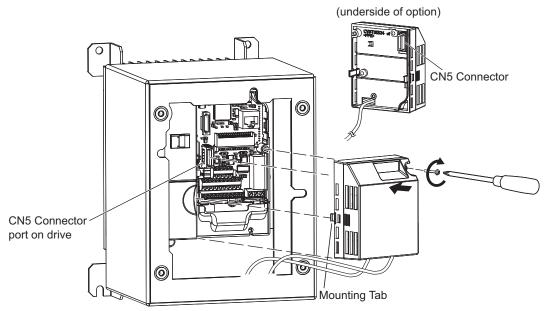
Figure 36 Attach Option Unit to Drive
