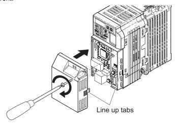
Figure 25 Attach the Option Cover
