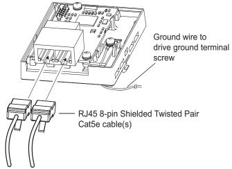
Figure 33 Communication Cable Ports
