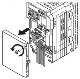
Figure 7 Remove the Front Cover
