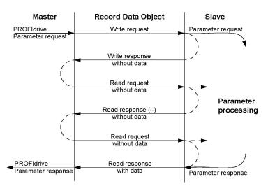
Figure 42 PROFIdrive Compatible Acyclic Parameter Access Mechanism Structure
