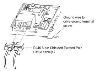
Figure 24 CN1 RJ45 CAT5e Communication Cable Ports
