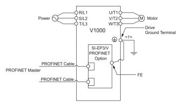
Figure 40 Wiring Diagram
