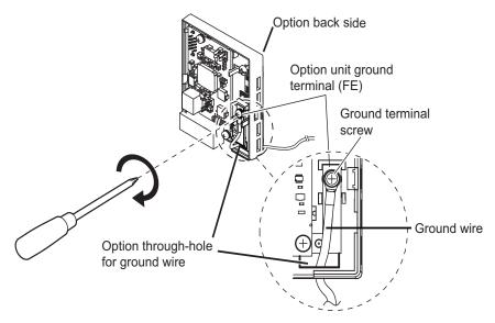
Figure 32 Ground Wire Connection Option Unit Side
