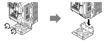
Figure 14 Remove the NEMA Type 1 Conduit Bracket
