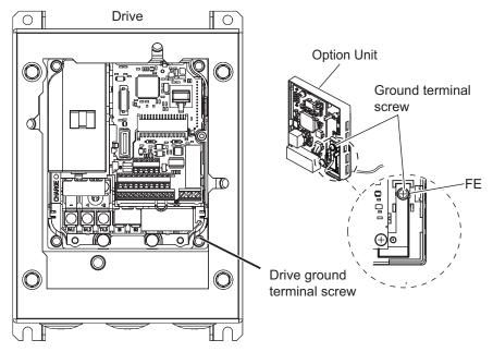
Figure 29 Remove Ground Terminal Screws
