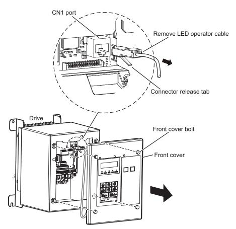
Figure 26 Remove the Drive Front Cover
