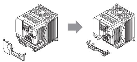
Figure 9 Remove the Terminal Cover and Bottom Cover on an IP20/Open-Chassis Drive (Models CIMR-V□□BA0006B to BA0018B; 2A0010B to 2A0069B; 4A0001B to 4A0038B)
