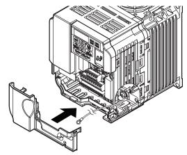
Figure 19 Reattach the Terminal Cover (Models CIMR-V□BA0006□ to BA0018□; 2A0010□ to 2A0069□; 4A0001□ to 4A0038□)
