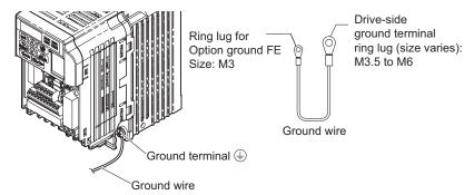
Figure 11 Ground Wire Connection on IP20/Open-Chassis
