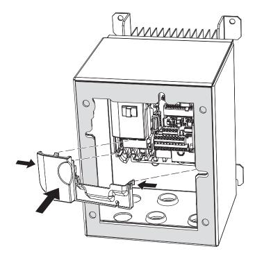
Figure 35 Reattach the Lower Terminal Cover
