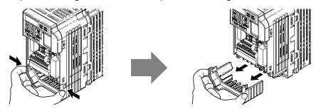
Figure 8 Remove the Bottom Cover on an IP20/Open-Chassis Drive (Models CIMR-V□□BA0001B to BA0003B and 2A0001B to 2A0006B)
