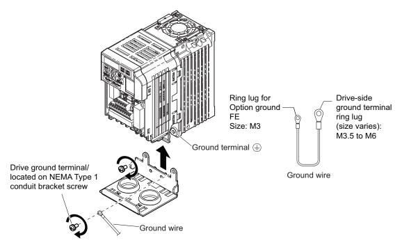
Figure 16 Reattach the NEMA Type 1 Conduit Bracket and Connect the Ground Wire
