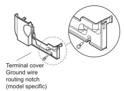
Figure 20 Terminal Cover Ground Wire Notch (Models CIMR-V□BA0006□ to BA0018□; 2A0010□ to 2A0020□; 4A0001□ to 4A0011□)
