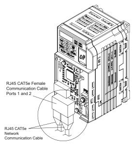
Figure 3 RJ45 Connections
