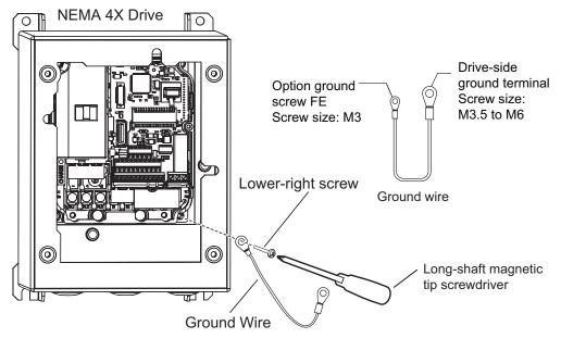
Figure 31 Drive-side Ground Wire Connection
