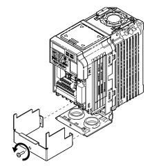
Figure 12 Remove the NEMA Type 1 Terminal Cover
