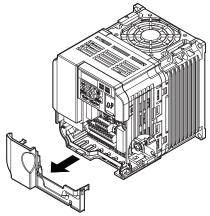
Figure 13 Remove the Terminal Cover on an IP20/NEMA Type 1 Drive (Models CIMR-V□BA0006F to BA0018F; 2A0010F to 2A0069F; 4A0001F to 4A0038F)
