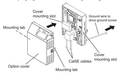
Figure 34 Attach the Option Cover
