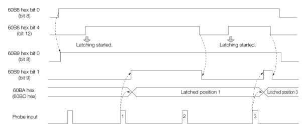
• Continuous Trigger Mode (60B8 hex bit 1 = 1 or bit 9 = 1)
