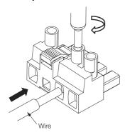
**6.** Connect the Dynamic Brake Resistor to the D1 and D2 terminals on the SERVOPACK.
