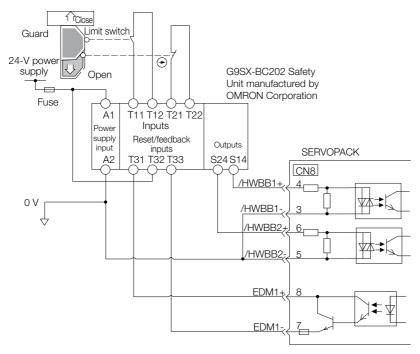
When the guard is opened, both the /HWBB1 and the /HWBB2 signals turn OFF, and the EDM1 signal turns ON. Because the feedback circuit is ON while the guard is closed, the Safety Unit is reset, the /HWBB1 and the / HWBB2 signals turn ON, and the operation is enabled.
