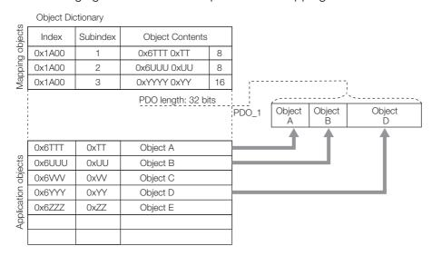
In addition to the above PDO mappings, PDOs have to be assigned to the Sync Managers to exchange EtherCAT process data.
