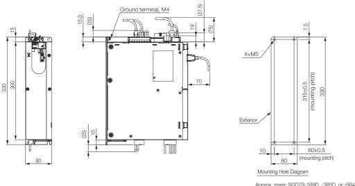
Approx. mass: SGD7S-1R9D, -3R5D, or -5R4D: 3.4 kg SGD7S-8R4D or -120D: 3.7 kg Unit: mm
