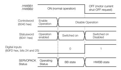
• When HWBB Operates While Power Is Supplied to Servomotor
