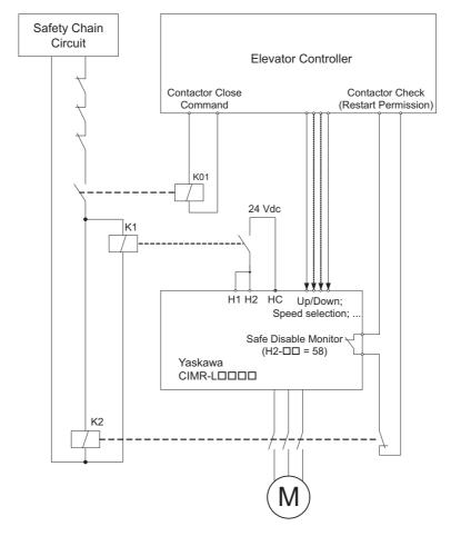
**Note: 1.** The drive output will immediately shut off when either of the inputs H1 or H2 is opened. In this case the brake should apply immediately in order to prevent uncontrolled movement of the elevator.
