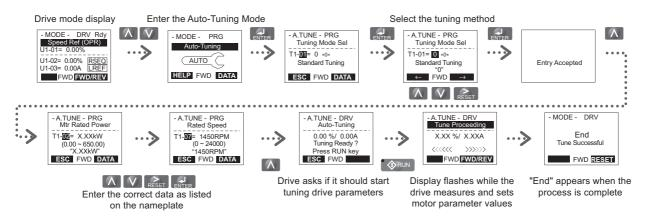
If Auto-Tuning cannot be performed for some reason (no-load operation impossible, etc.), then set the maximum frequency and voltage in the E1- $\square$  parameters and enter the motor data manually into the E2- $\square$  parameters for induction motors or E5- $\square$  parameters for PM motors. Refer to *Auto-Tuning Errors on page 46*.
