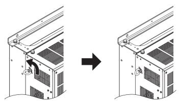
Figure 2 Adjusting Angle of Eye Bolts (CIMR-L□2□0346, 2□0415, 4□0216)
