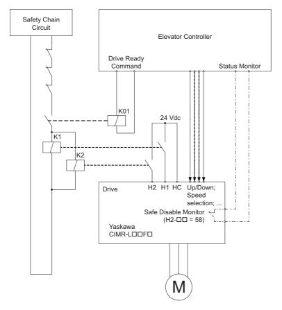
**Note: 1.** The drive output will immediately shut off when either of the inputs H1 or H2 is opened. In this case the brake should apply immediately in order to prevent uncontrolled movement of the elevator.
