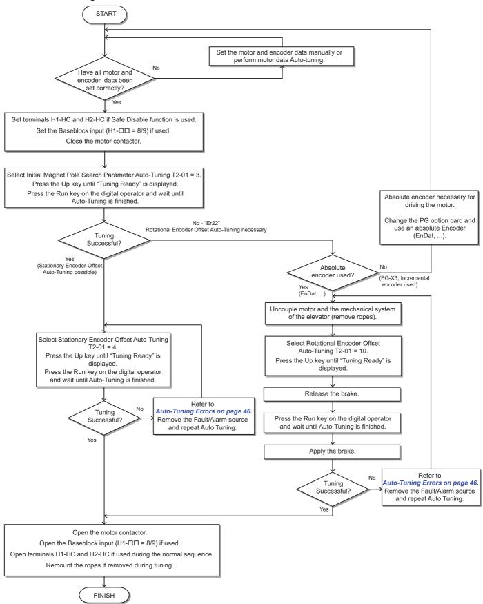
**Note:** When the first operation trial after non-rotating encoder tuning fails, e.g., due to wrong encoder rotation direction, repeat the encoder offset tuning after correcting the fault cause before starting a new trial.
