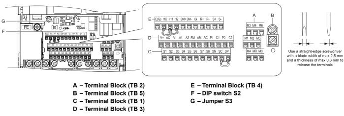
DIP switch S2 and jumper S3 are located on the terminal board. Set them as described below.
